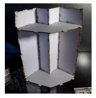
Attach lower internal frame piece thingy. Note : In photo above it's shown solid, the production piece has center cut out so you can install windows later if you like.
